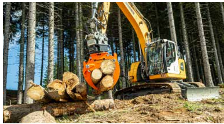
Gripper opening stroke 1270 mm.
