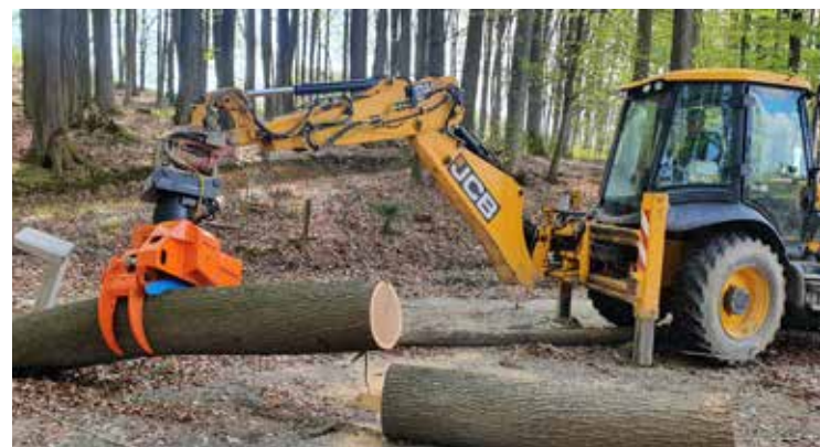
Sturdy and low-wear woodgripper with saw unit.
