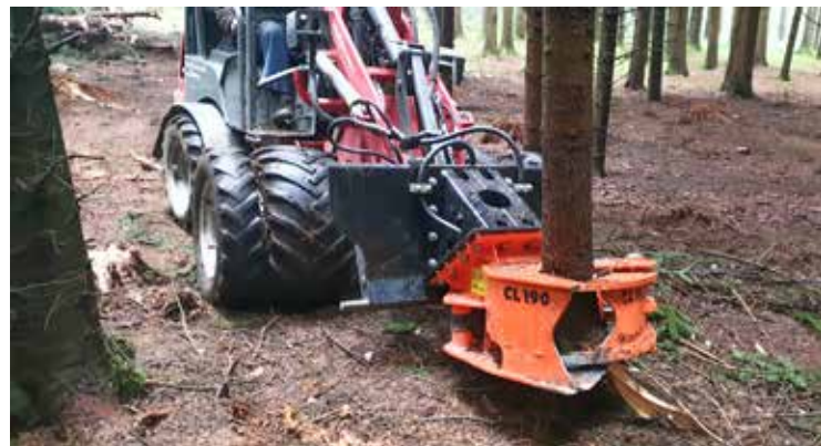
Woodcracker® CL190 cuts weak wood up to 25cm.
